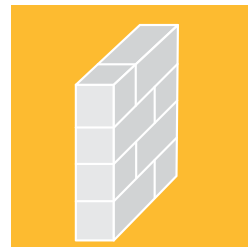
Perete exterior monostrat Ytong - 300 mm
